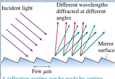
A reflection grating can be made by cutting parallel grooves in a mirror surface. These can be very precise, for scientific use, or mass produced in plastic.
