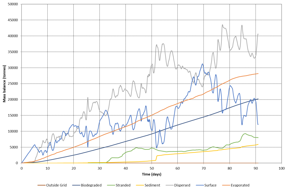
Figure 11.9: Mass balance of oil from well blow-out scenario throughout simulation
