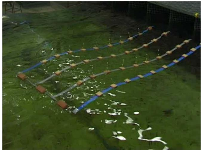
that uses optical fibres and signal processing to measure wave shape in tanks, as illustrated below.
