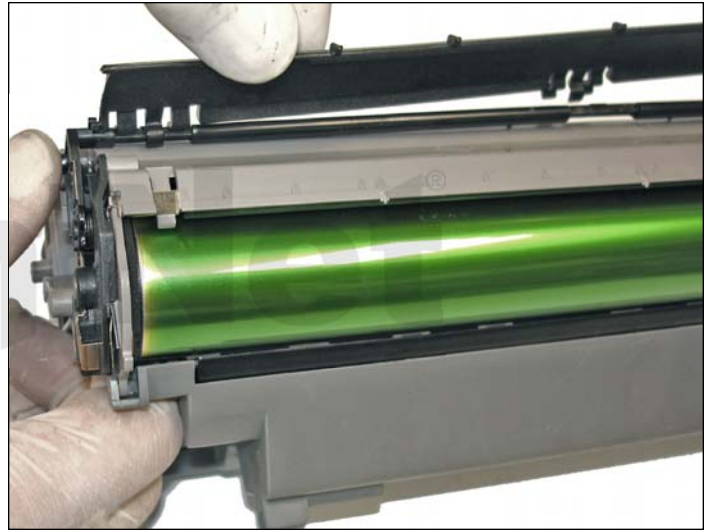
29. Carefully insert the drum shutter from the left side.
