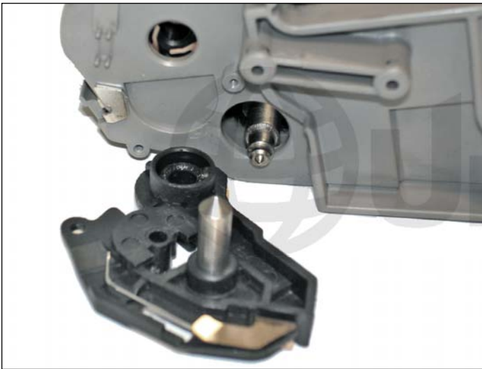
12. NOTE: The silver contact bar connected to the rear of the plate may come loose. Make sure it stays in it's original position as shown, for reassembly.
