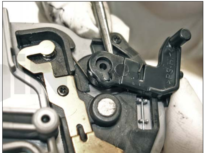
8. Using a small, flat head screwdriver, lift the drum shutter arm out from the connecting plastic pin to remove it. Do not lose the attached spring!
