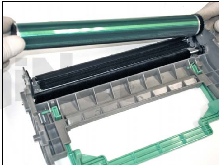
13. Remove the OPC drum, lifting from the left side.
