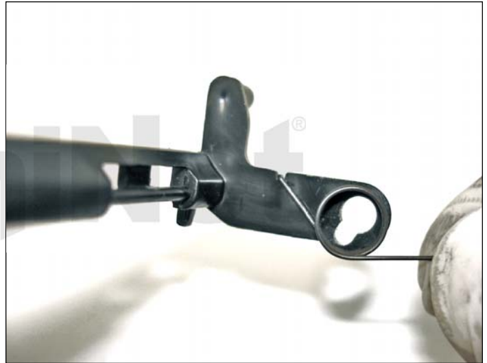
27. Attach the spring to the drum shutter arm.
