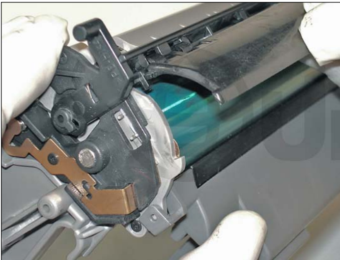
7. Remove the drum shutter, pulling from the contact side.
