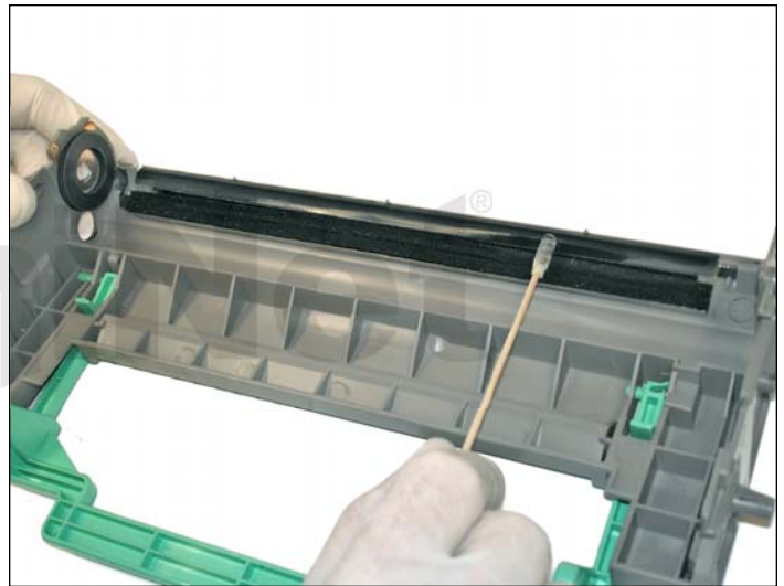
17. Clean the recovery blade using a clean cotton tip swab and isopropyl alcohol. Be careful not to damage or bend the blade! Doing so, will cause spotting.
