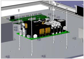
12. Using the 2 mm hex driver, carefully tighten the screws to secure the power supply.
