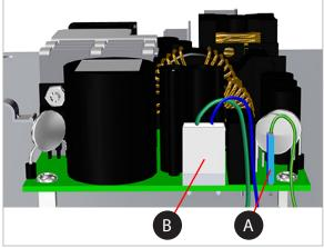
14. Using a Phillips screwdriver, reconnect the wire connectors to both the positive terminal and negative terminal using the original two (2) screws.
