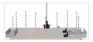
6. Lift the front edge of the floor and secure it through the slot to the front chassis crossbar with a zip tie.
