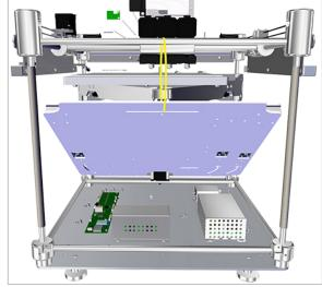
10. Using a 2 mm hex driver, loosen and remove the four (4) screws securing the power supply to the standoff pems and remove the power supply.
