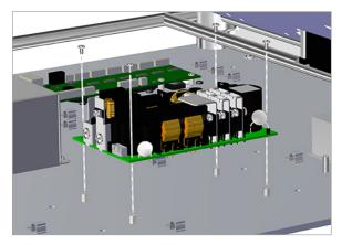
11. Place the new power supply over the standoffs and insert the original screws.
