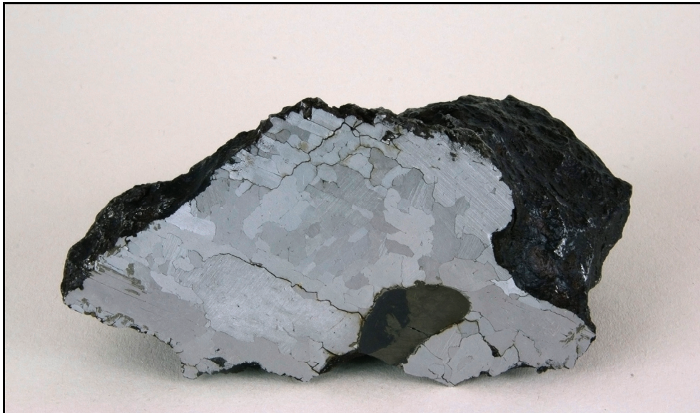
Polished and etched surface of the Morasko meteorite with coarse-grained intergrowths of kamacite and taenite. A rounded graphite-troilite nodule is visible in the lower part (troilite – brown, graphite – dark grey); length of the section – 13 cm
