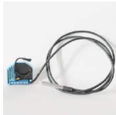
Temperature sensor connection to the module
