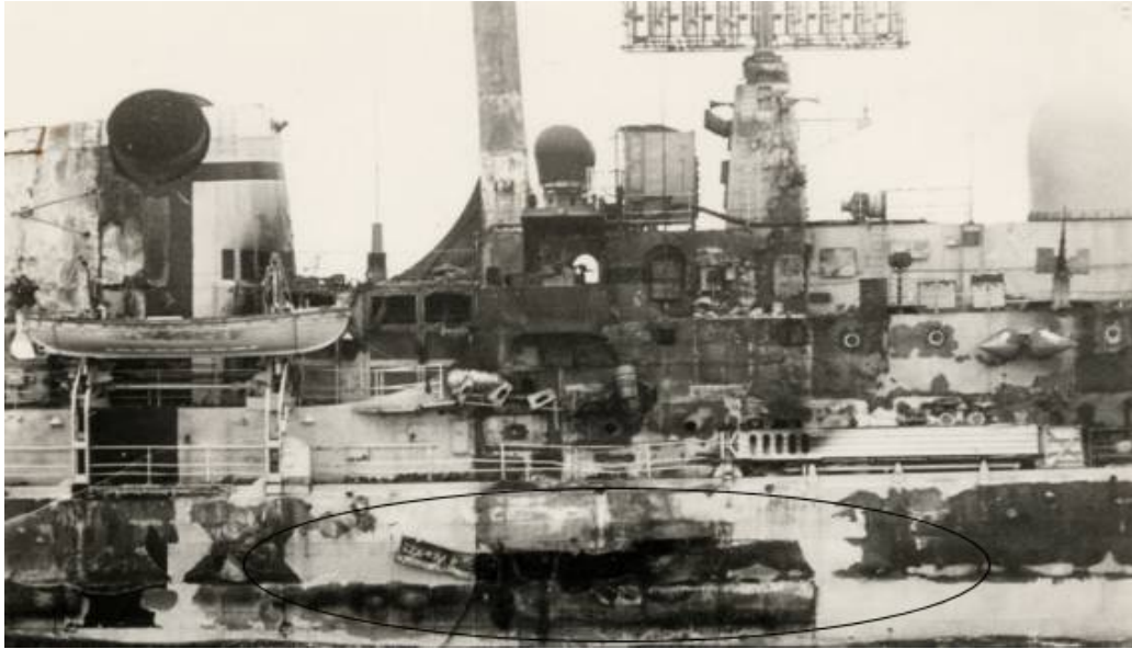
Above: Starboard side of HMS SHEFFIELD showing the hole made by the Exocet
