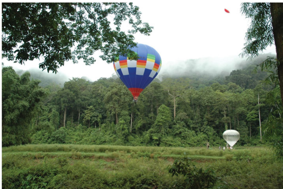
FIG. 3. The cinébulle (the coloured hot air balloon with a small propeller engine) in flight, and the Bulle des Cimes (the white helium balloon) on the ground. Between the two balloons is a rope attached to the tree crowns on which the Bulle moves.
