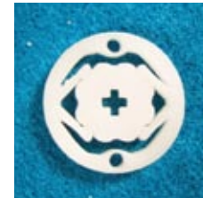
An indexing clutch protects the servo from excessive torque. It feels different than normal recording if it slips. It also allows a position to be easily recovered.
