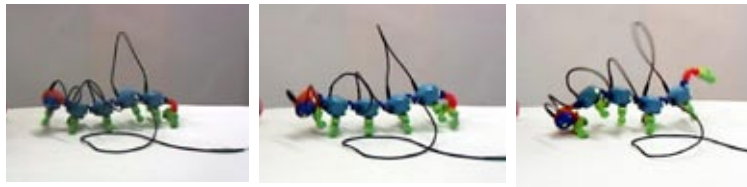
This caterpillar has been built to explore principles of phase shift and wave propagation.
