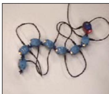
With Topobo, children can create wave-like motions by combining Queens (same motion everywhere) with the Time Delay Backpack.
