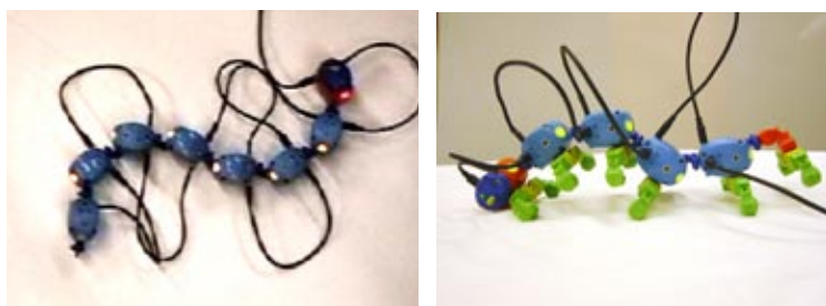
Distributed Time Delay leads to waves (left) and a walking caterpillar (right).
