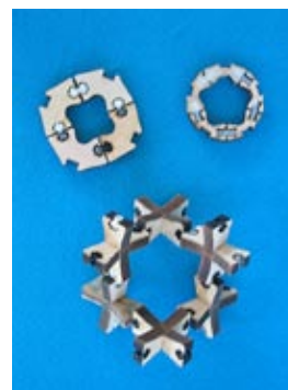
The first generation of parts were laser cut from bass wood and outfitted with LEGO connectors.
