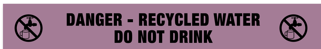
Figure 17 Example of warning tape laid above buried pipe that reticulate recycled water. Tape meets Aust standard being a minimum of 75mm wide and stating "Recycled water" and "Do not drink".
