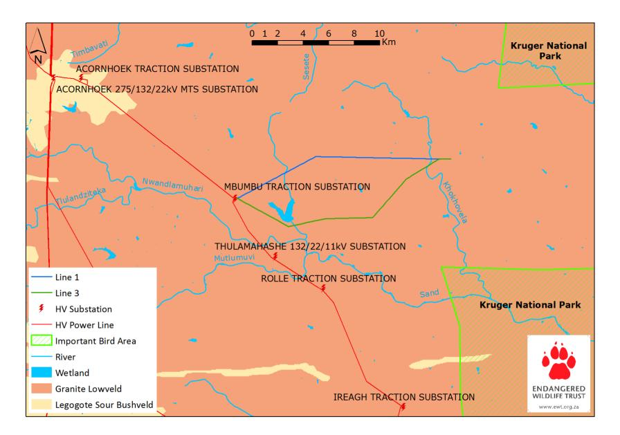
Figure 1: Map indicating the proposed project power line route options, existing high voltage electrical infrastructure, IBA's, rivers and the vegetation classification for the broader study area according to Mucina & Rutherford, 2006.
