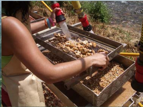
Washing-screening and sampling field lab next to the Arlanzon River
