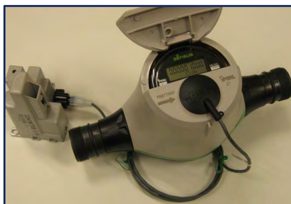
Secondary Water Meter with Radio Transmitter Source: Weber Basin Water Conservancy District
