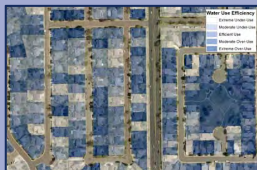
Water Use Efficiency Map – Parcels can be analyzed and displayed by water use efficiency
