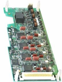
The CN3 connector provides connection to 4 analog station ports and are not polarity sensitive. The 4SLIDB is installed on the 4SLIU PCB. Up to 2 PCBs can be installed in the system maximum, but this number may be reduced depending on how many 4SLIU PCBs are installed. If 3 4SLIU PCBs are installed, only 1 4SLIDB can be installed. If 4SLIU PCBs are installed, the 4SLIDB can not be used.
