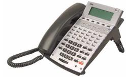
The 34-Button Aspire IPPhone has a 3-line, 24-character display with four interactive soft keys for intuitive feature access. In addition, it has 24 user-programmable function keys (with Dual LEDs) for one-button access to co-workers, features and outside lines. The telephone also provides 10 user-programmable One-Touch (Personal Speed Dial) keys and 15 additional fixed feature keys.
