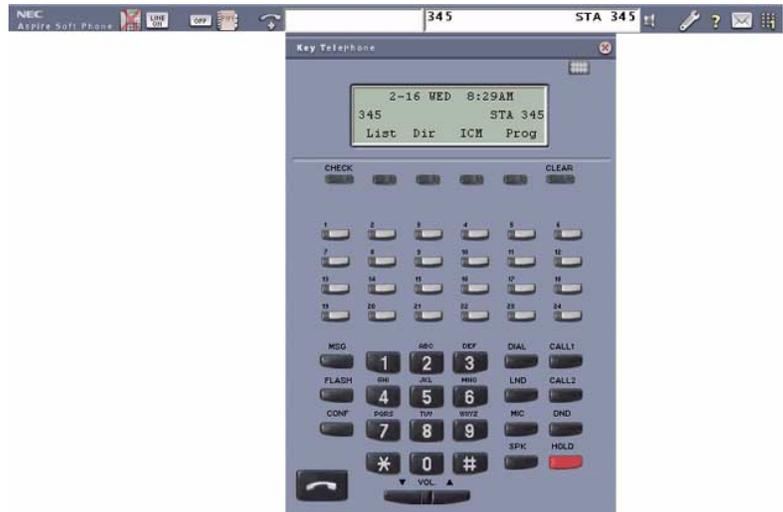
The Aspire Soft Phone delivers high quality voice via a USB-connected handset or headset or via a PC sound card, microphone and speakers. The Aspire Soft Phone functions include, not only making and receiving calls, but also placing calls on hold, intercom calls, conferencing, etc. The application can display a layout of an Aspire keyset to allow for ease of operation. Using the cursor, simply point and click to operate the Aspire Soft Phone as you would an Aspire keyset.
