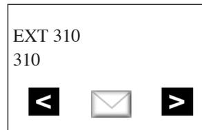
If the Aspire Wireless is out of range or if the phone is turned off, the message indication will be delayed until the phone returns into range or is powered up.
