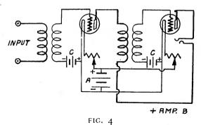
Showing how the C battery is connected in an audio-frequency amplifier
