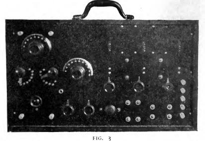
A portable three tube Grimes set, for outside antenna or loop, built by Mr. Searing
