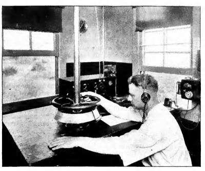
A RADIO COMPASS RECEIVING STATION At Sandy Hook, N. J. The operator is shown turning the wheel which adjusts the position of the big loop aerial. This station is connected by land wire to the control station shown on page 274
