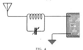
One method of connecting parts of a "wave-trap"
