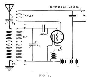
Diagram for a three-coll honeycomb set. For best operation, the primary, secondary, and tickler coils should be comparatively large, the tuning being done with condensers  $C_1$  and  $C_2$ , the latter should be of small capacity, as outlined under "undesirable effects of capacity"
