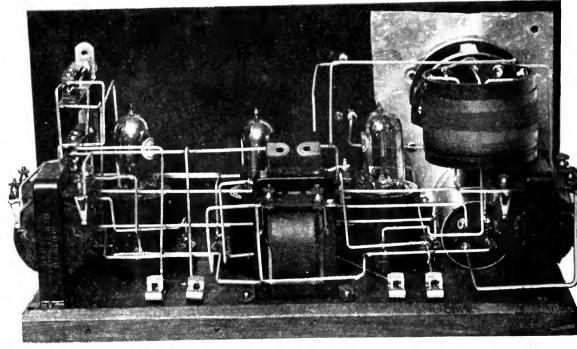
FIG. 4 Rear view of the completed set. Note the neat wiring, and the partial shielding
