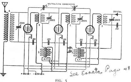
The best Inverse Duplex circuit we have yet seen. The neutrodyne condenser helps smother self-oscillations
