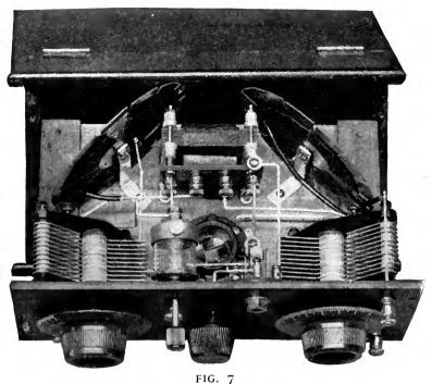
The "works" of Mr. Brown's one tube reflex set. Note the spider-web coils
