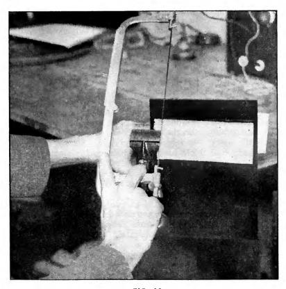
FIG. 10 Making a long cut with a hacksaw, the blade turned sideways
