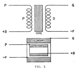
Showing the audio-frequency transformer connections
