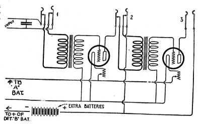
FIG. 2 The circuit of Fig. 1 with jacks added
