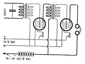
FIG. I The circuit submitted to The Grid
