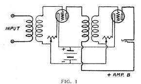
Two-stage audio amplifier. If the transformers are of reliable make and matched for the tubes, any distortion must occur in the tube circuit
