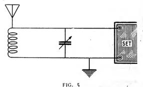
This arrangement is more efficient in cutting out spark interference than that of Fig. 4
