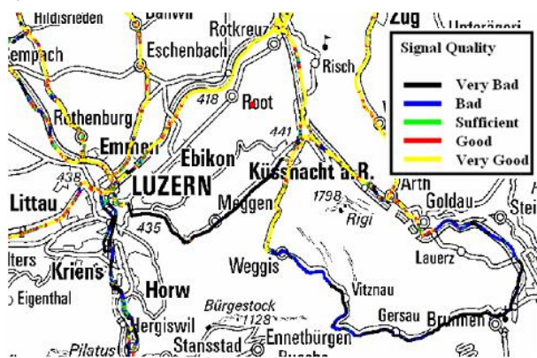
Fig. 4: Digital coverage at the fringe and outside of FM analog coverage area. In strong multipath areas (like the sections with the black color on analog graph) there is much better digital than analog coverage.
