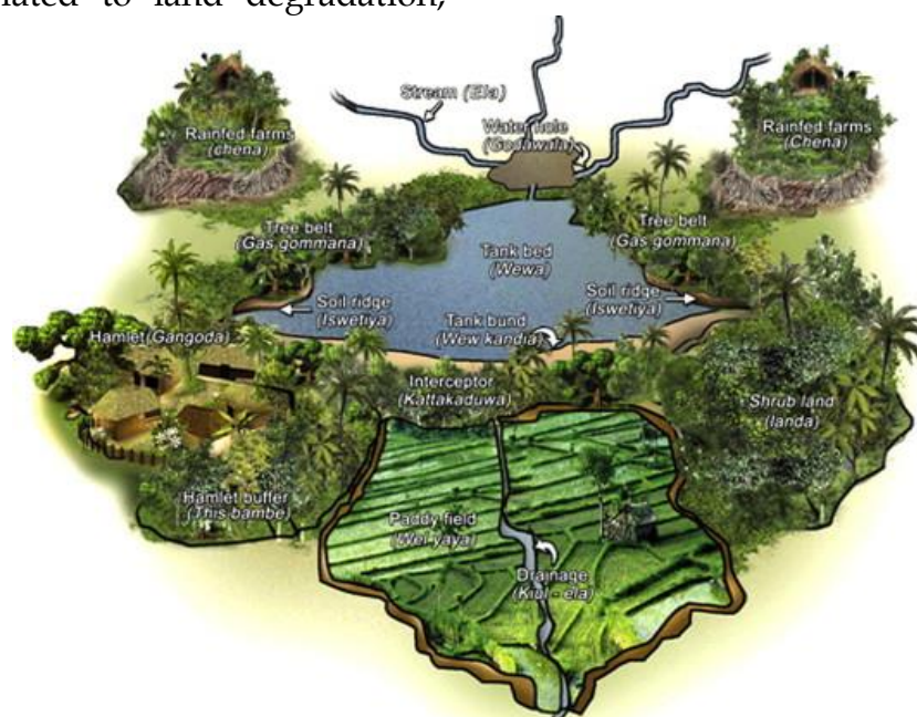
Figure 5.1. Components and their relative positions in the small tank system in Sri Lanka (Dharmasena 2010)
