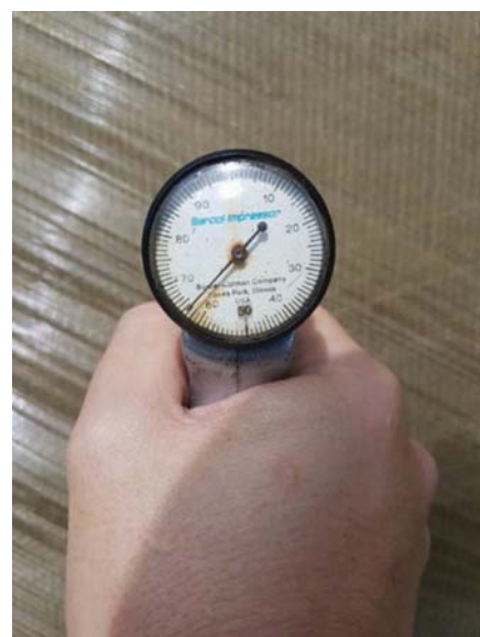
Figure 5—Barcol test on a new duct
