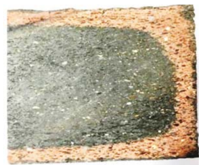
Figure 1 – Cut section of a red acid brick
