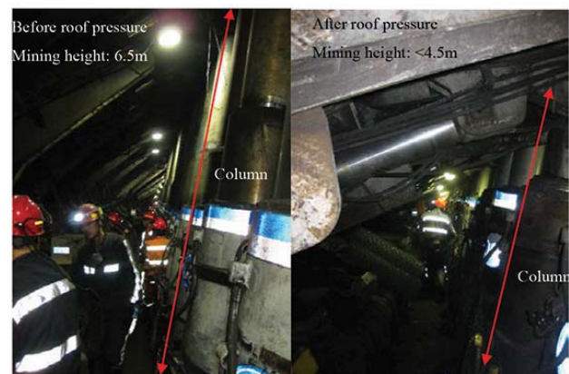
(c) Comparison of mining height before and after roof pressure
