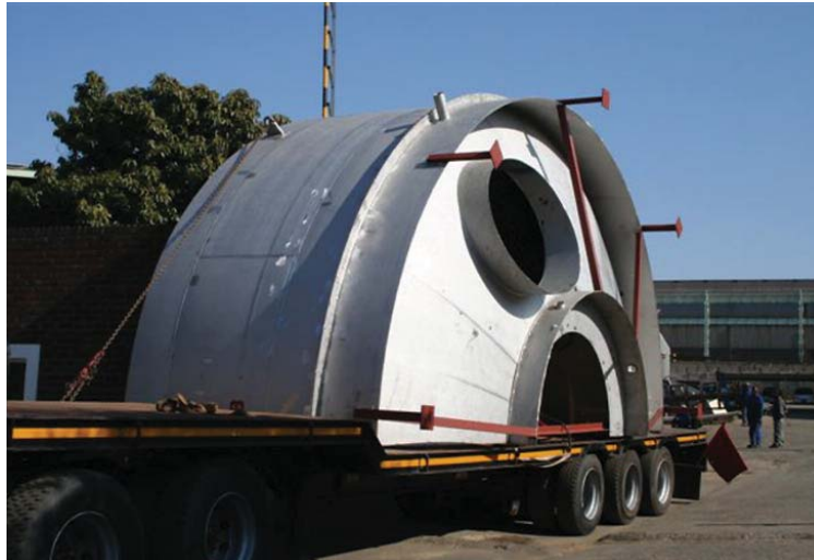
Figure 7—Prefabricated converter modules
