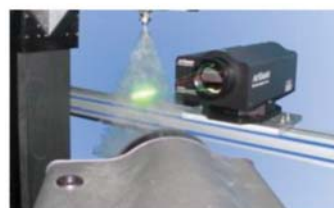
Figure 3b—PDI testing set-up
