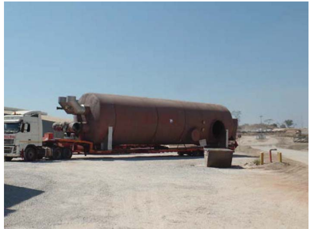
Figure 4—Sulphur furnace shell delivered to site
