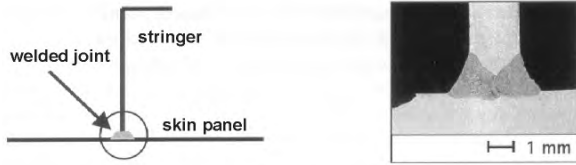
Figure 11. Laser-beam welding of a skin-stringer joint (cross section) [8]
