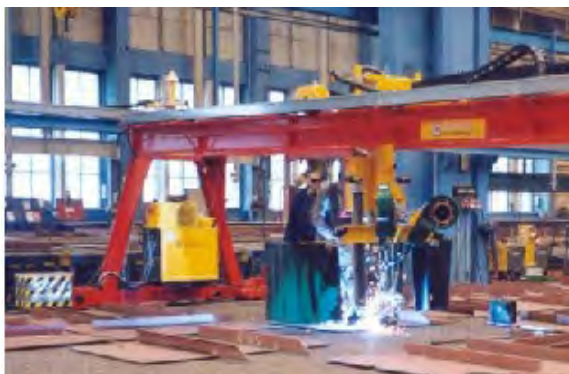
Figure 9. MAG flat-wire welding process for the production of profile welding
