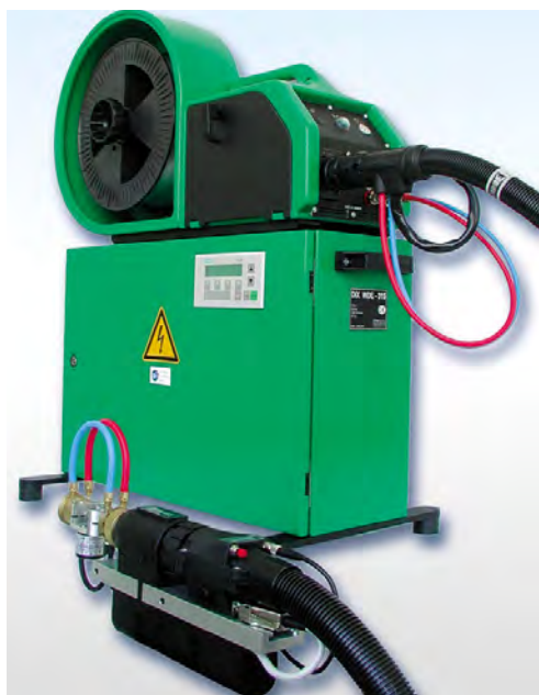
Figure 2. Dinse wire-feed system, complete with two drive units (PUSH-PUSH operation)
