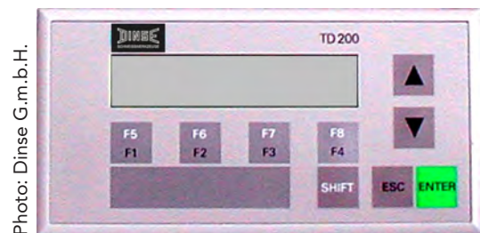
Figure 10. Integrated display in Dinse's wire-feed module for controlling and viewing process variables during laser-beam welding.
