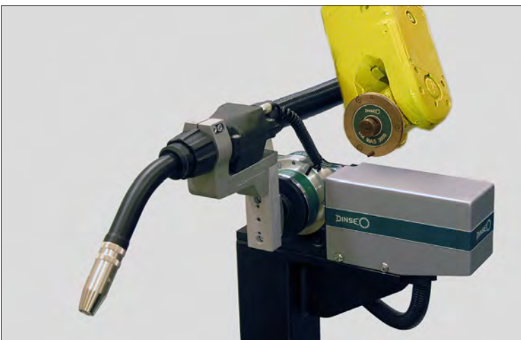
Torch system in the storage station uncoupled from robot
