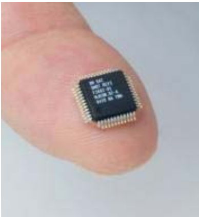
The XM “Connect-and-Play” chip makes a wide variety of home entertainment systems capable of receiving XM Satellite Radio.
