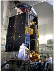
The EADS Astrium-built satellites for Inmarsat's new mobile communications Broadband Global Area Network are larger and more powerful than any other geomobile satellites (EADS Astrium/ C. Mériaux photo)
