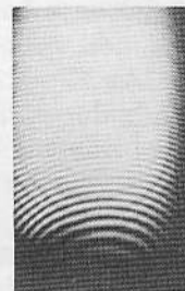
Fig. 27. Interference fringes seen with the Interferometer of Figure 26.
