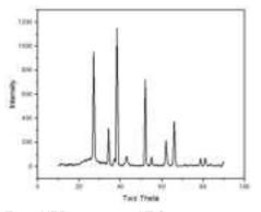
Fig. 7 XRD spectrum of TiO<sub>2</sub>
