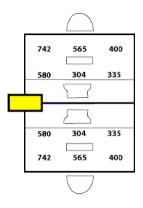
Direct-indirect stand alone luminaire. Its independence with the ceiling allow to locate the luminaire very precisely near the work space. The users appreciated the dimming option associated to the daylighting-occupancy sensor. Can be shared with another occupant. Considered as high standing. Typically 100W per work space required, less than 8W/m² in open plan office. Typical light sources about 2 CFL 55W per occupant, partly dimmed.
