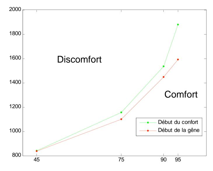
Relative position of luminaire (angle of vision)
