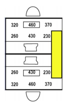
Direct-indirect suspended luminaire. Allow usage of 1.20 or 1.50m fluorescent tube. But work place cannot move if luminaire position is fixed. Leads to the lowest electrical consumption: 6W/m². In open plan office. Could use 2x54 W fluorescent tubes for two people.
