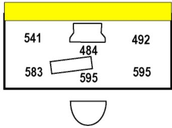
Indirect luminaire integrated to the furniture. Juged as very comfortable, the ceiling luminances are moderate, but the general feeling tends to have a work plane looking darker that the rest of the room. Requires about 2x35 W fluorescent tubes per work place.
