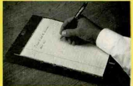
Using a digital pen equipped with an RF transmitter, you take notes on a standard 8 1/2" × 11-inch lined notepad affixed to the *CrossPad's* digital notepad. Meanwhile, signals from the digital pen are stored as digital notes in the pad's memory. The keyword feature allows you to circle a word and search for it later, making it easy to retrieve your notes. Change pages by flipping the page over.
