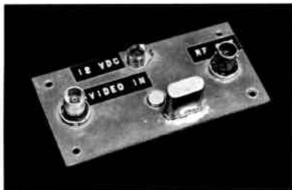
Heart of the ATV system is the LP-2000 IC next to the crystal.
