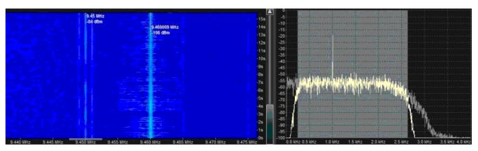
Shows E25 carrier with 1kHz tone[left], and audio response, right
