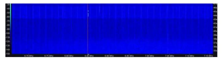
The red line designates the frequency. Strangely the actual message transmission was very weak, inaudible in places. There was little or no QRM on 6846kHz and one has to ask if the signal weakness is due to the vagaries of propogation or what.
