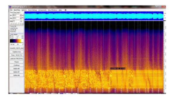
Usually there is nothing unusual or unique to see in many of the transmissions, but in this example at an audio frequency of 2.031880 kHz you can see throughout the transmission a line (spurious carrier?) in the trace, above the CROWD36 tones. Is this unique to this transmitter? If it is then any further signals showing the same characteristic are likely to be from the same transmitter.
