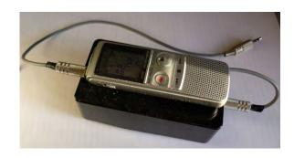
Battery box below the recorder holds two D Cells.
