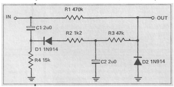
Because of component availability I now use for C1 and C2 2u2 tantalum whilst D1 and D1 are 1N4148 diodes. I cannot recall where I discovered the circuit but all credit to its designer.
