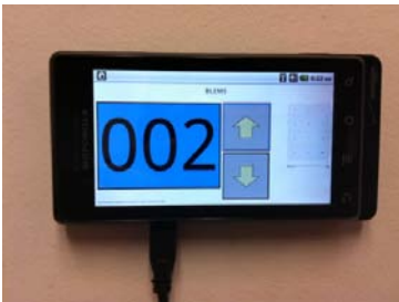
Figure 4. Mobile device used to collect occupancy ground truth.
