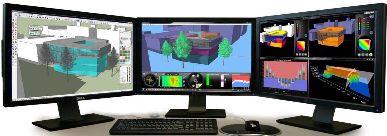
Figure 9. The prototype implementation allows a single user to simultaneously model, simulate, and view BES results. The workstation's left screen shows the CAD input, while the center shows the translated model and the right contains BES output.
