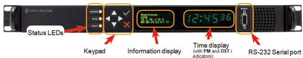
Figure 4-1: SecureSync front panel
