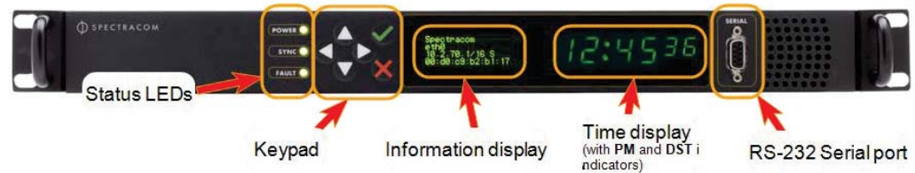
Figure 2-1: SecureSync front panel
