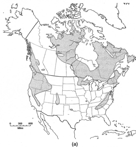
Figure 6.16. Lake Acidification in North America. (a) Regions in North America containing lakes that would be sensitive to potential acidification by acid precipitation (shaded areas). These areas have igneous or metamorphic bedrock geology which results in dilute lakes with low \text{HCO}_3^- concentrations ( <0.5 \text{ mEq HCO}_3^-/\text{l} ). Unshaded areas have calcareous or sedimentary bedrock geology. (From J. N. Galloway and E. B. Cowling, "The Effects of Precipitation on Aquatic and Terrestrial Ecosystems, A Proposed Precipitation Chemistry Network," Journal of the Air Pollution Control Association 28(3): 233. Copyright © 1978. J. of the Air Pollution Control Assoc. Reprinted by permission of the publisher.)
