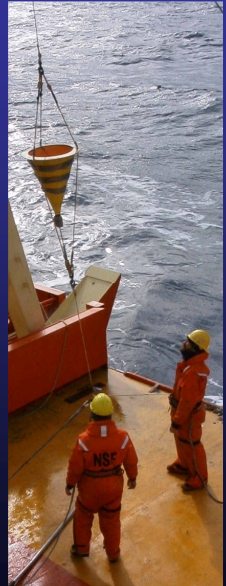
SEDIMENT TRAP RECOVERY
