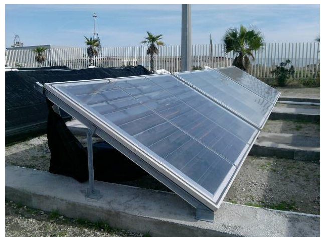
Figure 7.7 AOSOL CPC solar collector developed for the MEDESOL project
