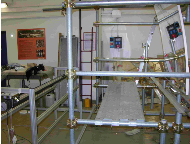
Figure 5.7 VISprofile . The linear array of point light sources is placed along the focus of a parabolic-trough panel. On the left, not shown, the camera is installed on the translational rail.
