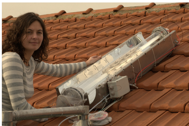
Figure 7.15 Photocatalytic reactor for the treatment of real polluted air from a wastewater treatment plant.
