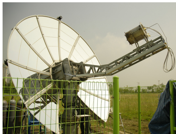
Figure 4 5. Solar Dish System (INHA-DISH1) with 5-kW th absorber used for CO_2 reforming of methane.
