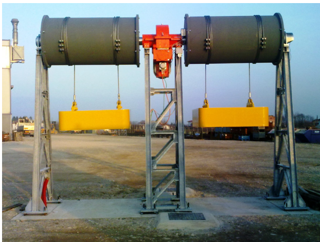
Figure 5.9 D.D. tracking drive: testing drums
