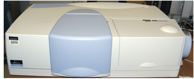
Figure 5.28 Perkin Elmer Lambda 1050 Spectrophotometer in the solar reflector test laboratory
