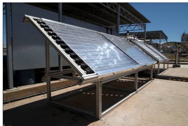
Figure 7.14 Glass tube photocatalytic reactor in the focus of Compound Parabolic Collector.
