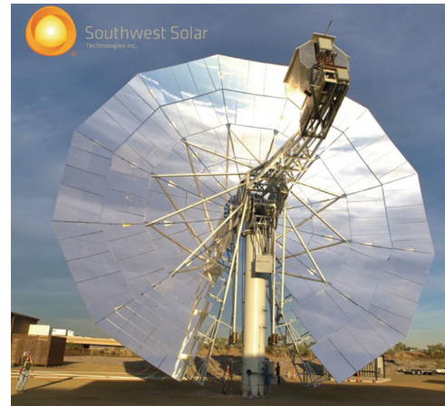
Figure 5.15 SouthWest Solar Technology dish with Brayton Energy PCU
