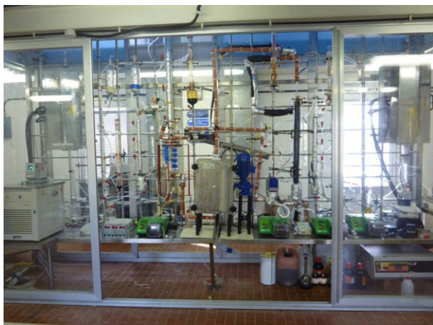
Figure 4 15. Testing performed in SI lab scale plant ( 10 \text{ l}_N \text{ H}_2 / \text{h} ) at ENEA's Casaccia Research Centre, Italy.
