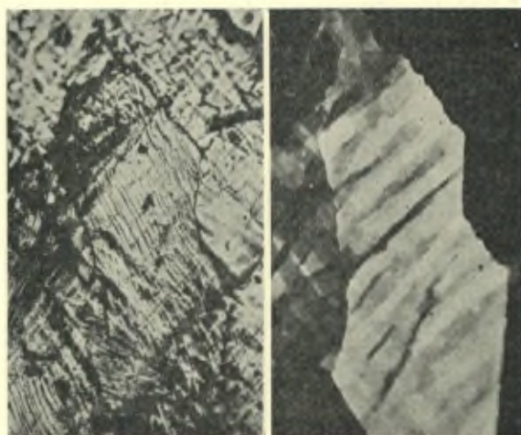
Fig. 2. — Creep specimen extended 31 %, × 100 Left — deformed surface. Right — same field, section just below surface.
