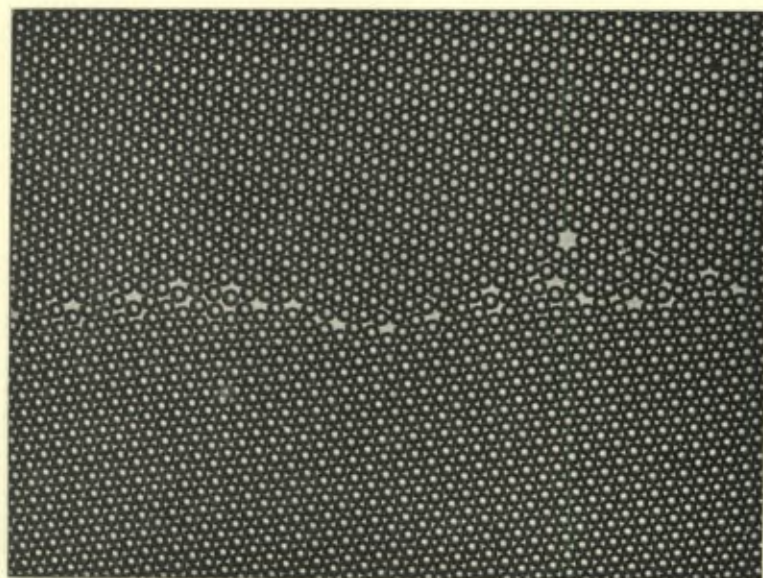
Fig. 3. — Boundary between regions disoriented by 25°.
