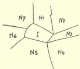
Fig. VII, 9. — Schematic representation of grain growth in a texture. It is assumed that the disappearing crystal I forms high-energy boundaries crystals N, while the crystals N form with each other low-energy grain boundaries. (After Rathenau and Baas, 1951).
