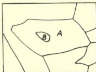
Fig. VII, 6. — Pear-shaped crystal ( B ) inside a large crystal ( A ). Both crystals are grown by primary recrystallization in fine-grained aluminium plate, the rate of growth of A was larger than that of B . About natural size. (After Burgers, 1947).
