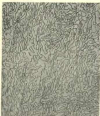
9.7 % Nickel alloy transformed at 650 °C. × 750
