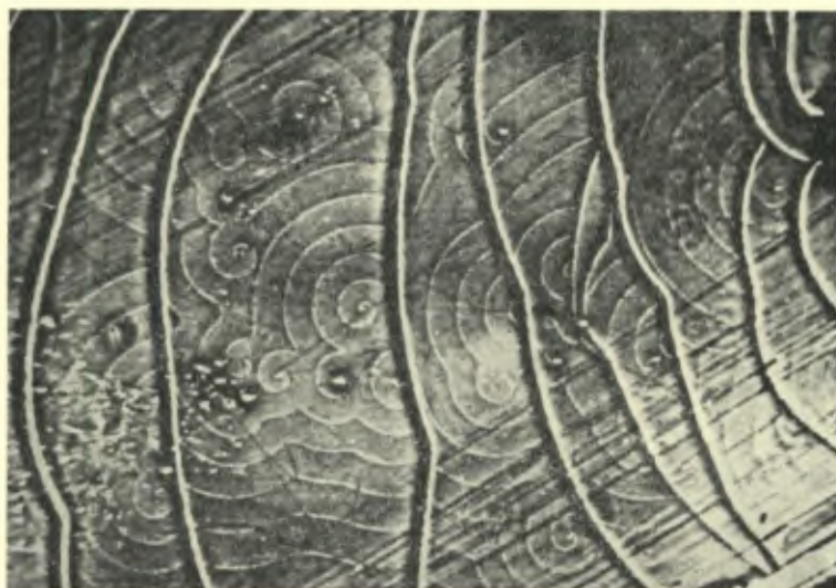
Figs. 7-10. — Growth steps on Carborundum, SiC (Verma).
