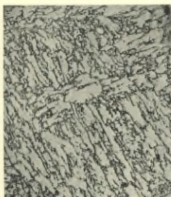
19.7 % Nickel alloy transformed at 450 °C for 1000 hours. Reaction still incomplete. × 750
