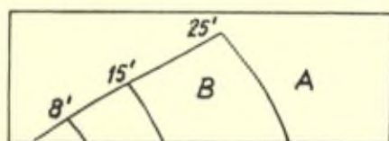
Fig. VII, 1. — Directional growth of a new crystal ( B ) in a stretched single crystal ( A ) of aluminium. The boundary position is indicated after 8, 15 and 25 minutes of heating at 600 °C. About natural size. (After Burgers and May 1945).
