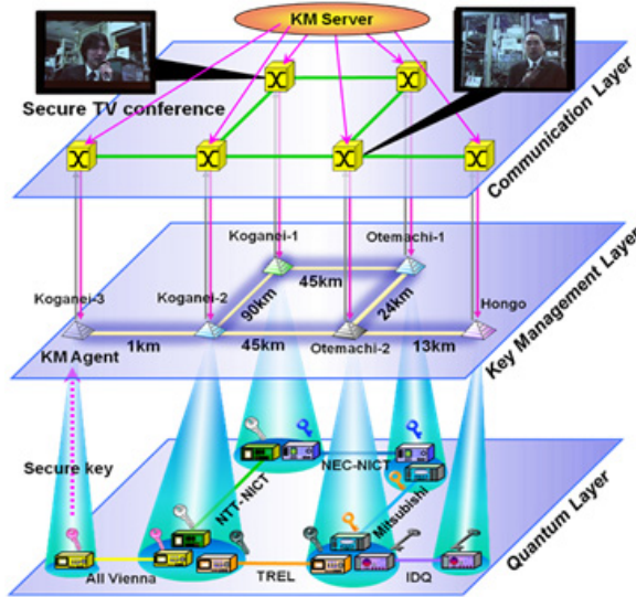
Fig. 2. Layout of the quantum cryptography network test in Tokyo (Sasaki et al. ).
