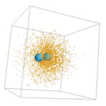
Chemically powered nanomotors are studied since about a decade in laboratories worldwide and are of both fundamental and applied interest. They are colloidal devices with a catalytic activity that enables them to harness a source of chemical energy to provide rotational or translational motion.
