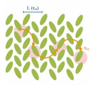
Figure 1. Schematic picture of charge transport in organic semiconductors. Charge are delocalized over a certain length-scale,  $L(\tau_{in})$ , below a given time-scale,  $\tau_{in}$ .
