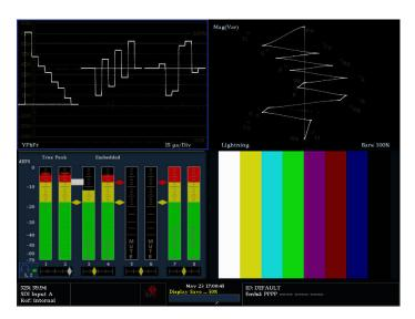
Composite Gamut compliance without the need for a separate encoder. Within this display, a separate upper and lower luma-only Gamut limit can be applied. This display is very useful for camera balancing.
