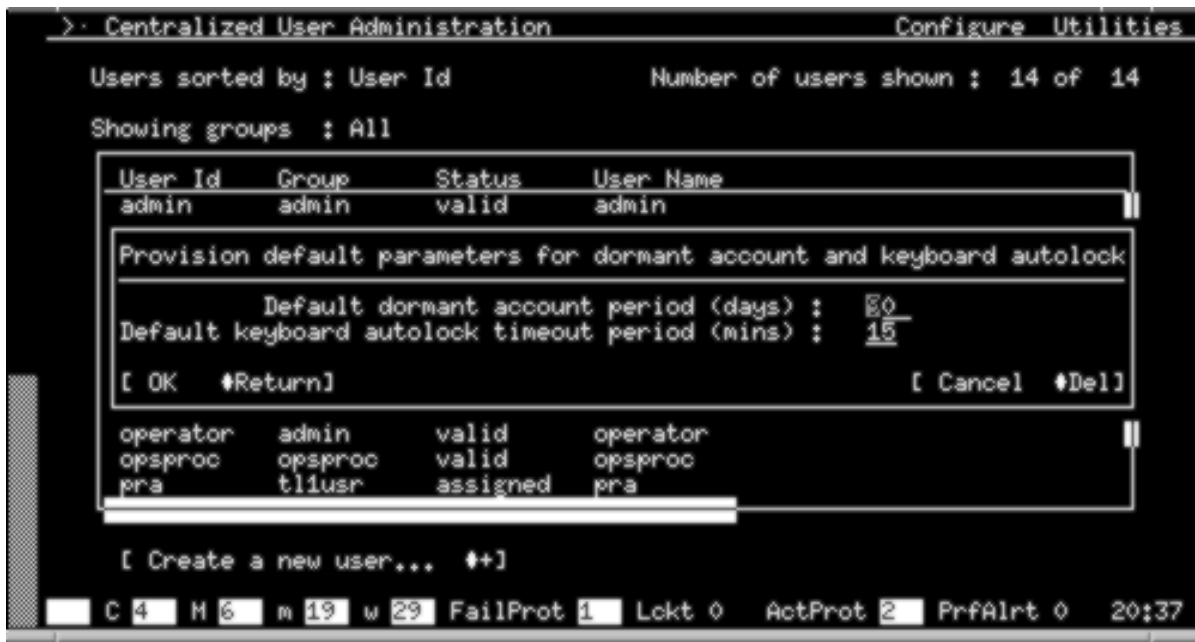
Figure 61 Provision to change the default values for dormant accounts and keyboard autolock-out
