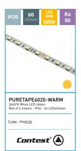
Monochrome adhesive ribbon of 300 warm white LEDs for 5m Width: 10 mm Colour temperature: 3000°K Luminosity: 915 lumens/m Power required: 14.4W/m (72W for 5m) Voltage required: 24V (+ and -) Cuttable every 10 cm (6LEDs) IP20: no protection no sealing
