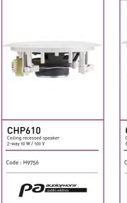
Power rating: 10 W RMS Available power: 10 W / 5 W / 2.5 W at 100 V Tweeter: 1.5 inch Woofer: 6.5 inch Frequency response: 56 Hz – 20 kHz Sensitivity (1 W (Q 1 m): 93 dB External dimensions (diameter and depth): 230 x 90 mm Drilling diameter: 200 mm Net weight: 1.4 kg
