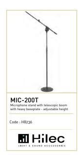
Microphone stand with telescopic boom with heavy baseplate Net weight: 5.3 Kg Height: from 92 cm to 1.52 m Baseplate diameter: 25.5 cm Thread at the boom tip: 3/8" Boom length: 55 to 90 cm Materials: - Aluminium for the boom hinge - Steel for the tubes and baseplate - Rubber for the ends of tubes - ABS for the knobs and the boom tip Finish: matte black epoxy paint
