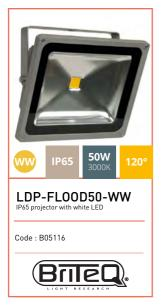
Optics: 1x50W 3000K COB LED Opening angle: 120° Power supply: 100-240V/50-60Hz Power consumption: 50W Waterproofing level: IP65 Natural convection cooling Finish: cast aluminium, painted white Dimensions: 290 x 236 x 150 mm Weight: 3.52 kg
