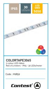
Trichromatic adhesive ribbon of 150 RGB LEDs for 5m Width: 10 mm Luminosity: 255 lumens/m Power required: 7.2W/m (36W pour 5m) Voltage required: 24V (+ and -) Cuttable every 16,8 cm (6 LEDs) IP65: Upper molded silicone dome
