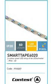
3-colour adhesive ribbon of 300 RGB LEDs for 5m pixel version Width: 10 mm Power required: 14.4W/m (72W for 5m) Voltage required: 5V DC Cuttable every 1.6 cm (1 LED) IP20: no protection no sealing
