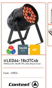
18x3W RGB LEDs Beam opening: 40° Light intensity: 1150 Lux at 3 m Infrared remote control Digital display with drop-down menu Input and output on IEC plugs Modes of operation: 2-6 channel DMX, Fixed colours, Step or Fade programs, Auto mode with sound sensitivity, Slave mode, Power consumption: 60 W Power supply: AC 100/240V - 50/60Hz DMX input and output Black aluminium housing Dimensions: 340 x 270 x 220 mm Net weight: 4.3 kg
