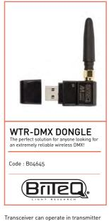
or receiver mode - 2.4 GHz frequency band Compatible with the "Wireless Solution" W-DMX<sup>™</sup> Protocol Works perfectly with Briteq WR-DMXG4 (4632) in WT-DMXG4 (4633) 5V DC power supply via USB port DMX connection via USB port Dimensions: 71 x 42 x 11 mm Net weight: 0.02 kg
