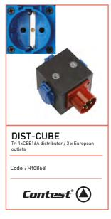
Cube format distributor 2 M10inserts Tetra CEE 16A input plug 3 16A standard German plugs (1 outlet per phase) Dimensions: 160 x 136 x 102 mm Weight: 0.86 Kg
