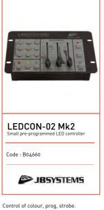
Fixed patch R,G,B, Dimmer/Strobe Works in 4 or 8 channel mode Power supply: DC 9-12V 300mA Dimensions: 210 x 140 x 46 mm Weight: 1 Kg
