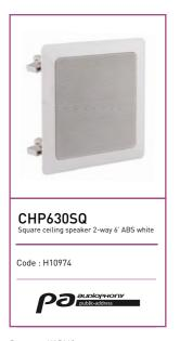
Power: 30W RMS Available power: 100 V 8 Ohms Components: 5" + 0.5 Sensitivity (1W/1m): 89 dB, +/- 3dB Frequency response: 90-20 000 Hz Construction: White ABS body Hook: 4 screwed tabs Dimensions: 220 x 220 x 220 x 95 mm Weight: 980 g
