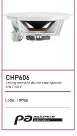
Power rating: 6 W RMS Available power: 6 W / 3 W at 100 V Speaker: double cone 6.5 inches Frequency response: 110 Hz – 13 kHz Sensitivity (1 W @ 1 m): 90 dB External dimensions (diameter and depth): 230 x 90 mm Drilling diameter: 200 mm Net weight: 0.9 kg
