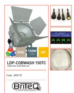
Optics: 1x150W RGB COB LED Opening angle: 60° Infrared remote control Integrated control unit with display with drop-down menu Waterproof wiring for power supply inputs/outputs and DMX inputs/outputs Power supply: 100-240V/50-60Hz Power consumption: 170W Waterproofing level: IP65 Natural convection cooling Finish: cast aluminium, painted white Barndoor included Dimensions: 326 x 344 x 220 mm Weight: 9.5 kg
