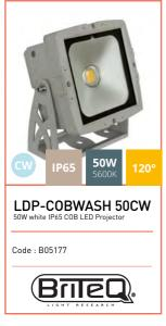
Optics: 1x 50W 5600K COB LED Opening angle: 120° Infrared remote control Integrated control unit with display with drop-down menu Waterproof wiring for power supply inputs/outputs and DMX inputs/outputs Power supply: 100-240V/50-60Hz Power consumption: 66W Waterproofing level: IP65 Natural convection cooling Finish: cast aluminium, painted white Barndoor option available Dimensions: 223 x 202 x 122 mm Weight: 3.8 kg
