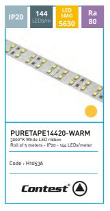
Double monochrome adhesive ribbon of 720 warm white LEDs for 5m Width: 20 mm Colour temperature: 3000°K Luminosity: 2452 lumens/m Power required: 47.5W/m [238W for 5m] Voltage required: 24V (+ and -) Cuttable every 8.4 cm [12 LEDs IP20: no protection no sealing
