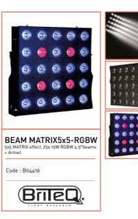
25 15W RGBW LEDs 5x5 Matrix Lens opening: 4.5° DMX mode: 4-150 channels Ethernet input/output: Art-Net support Internal programs in standalone mode or via DMX, Master/slave mode, static or fade colours, static or sound-triggered chasers. Halogen (slow) or LED (fast) mode Balancing of individual whites by Pixel Four intensity variation curves DMX IN/OUT on XLR 3/5-pin plug POWER IN/OUT with Powercon Power: AC 100 - 240V, 50/60Hz Power consumption: 415W Dimensions: 550 x 550 x 120 mm Weight: 18 kg
