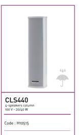
Power rating: 40 W RMS Available power: 40 W / 20 W at 100 V Speaker: 4 x 2.5 inches Frequency response: 250 Hz -15 KHz Sensitivity (1 W @ 1 m): 95 dB Aluminium body and grill, Ingress protection: IP44 (weather-resistant) Dimensions: 104 x 73 x 402 mm
