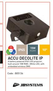
Optics: 1x15W RGBW LED Opening angle: 10° Wireless transmitter / receiver compatible with protocol W-DMX G4 Integrated control unit with display with drop-down menu Infrared remote control Power supply: 100-240V/50-60Hz Power consumption: 15 W Dimensions: 172 x 138 x 185 mm Weight: 1.61 kg
