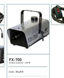
Heating element: 700W Preheating time: 5 minutes Tank: 0.8 litres Output volume: 70 m3/minute Wired remote included Wireless FC-5 remote optional Power supply: 230V - 50Hz Power consumption: 700W max. Dimensions: 330 x 160 x 130 mm Net weight: 3.65 kg
