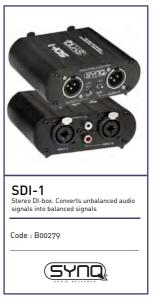
This stereo DI-box is the perfect solution for various applications! ' It allows conversion of unbalanced audio signals into balanced signals for transport through long cables. The "ground lift" switch allows separation of the inputs/outputs to avoid ground loops. Solid anodised aluminium black housing 1 RCA and XLR/6.35 jack combo input 1 XLR output Max. input level: +21dBu Dimensions: 105 x 110 x 44 mm Weight: 0.440 Kg
