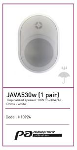
Power outputs : 15 / 30 W Voltage : 100 V 16 Ohms Components : 5" + 1" Sensitivity (1W/1m): 88 dB, +/-3dB Frequency response : 60 - 20 000 Hz Material : Plastic enclosure and aluminium grille Holding : Wallmount bracket Connectors : Waterproof cable on gland IP55 Power rotary knob : 30W 16 $\Omega$  // 15 / 30 W 100V Dimensions : 178x 236 x 255 (H) mm Weight : 2,38 Kg
