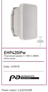
Power output: 2.5/5/10/20W Power supply: 100V 8 ohms Components: 4 +1Sensitivity (1W/1m): 88dB, +/-3dB Frequency reponse: 90 - 18,000Hz Material: white ABS enclosure and metallic grille Mounting: wall-mount yoke Connectors: waterproof cable on gland IP55 Power selector: 20W 8 $\Omega$  // 2.5/5/10/20W 100V
