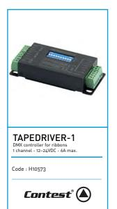
For monochrome ribbon DMX 1 channel 144W under 24V Dimmer by dip-switches Command in 0-10V control
