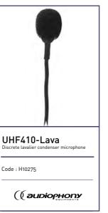
Miniature lavalier electret condenser microphone Sensitivity: -47 ±4dB Polarity: Omnidirectional cardioid Frequency response: 50Hz - 10KHz Operating voltage: 1.5V Power consumption: 0.5mA max. Signal to noise ratio: Higher than 58dB Accessories included: Windscreen and fastening pin Connectivity: Mini XLR Dimensions: 37 x 5.5mm diameter
