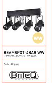
4 15W Warm white 3200K LED sources 4° opening per lens (10° and 45° filters included) Electronic dimmer variable from 0 to 100% 2 Mode dimmer: Slow (halogen), Fast (LED) 4 Dimmer curves (LINEAR, SQUARE, INV.SQUARE, S-CURVE) DMX mode: 1, 2, 4 or 5 channels Wireless DMX: WTR-DMX dongle (optional) Drop-down menu display to assign and select different modes DMX IN / OUT by XLR 3/5-pin plugs POWER IN / OUT by PowerCON plugs Spigot support 28mm Power consumption: 71W max.
