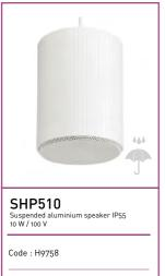
Power rating: 10 W RMS Available power: 10 W / 5 W / 2.5 W at 100 V Frequency response: 150 Hz – 15 kHz Speaker: 5 inch Sensitivity (1 W (a 1 m): 90 dB White aluminium body, Ingress protection: IP55 (weather-resistant) Dimensions (a x D): 138 x 205 mm Weight: 2.2 kg
