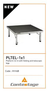
Material: Frame : Aluminium Tray: 12mm anti-slip plywood Dimension 1 x 1 m Thickness: 55 mm Telescopic legs from 40 to 60 cm high Permissible distributed load: 300 Kg/m². Finish: Aluminium / Black Weight: 18 Kg
