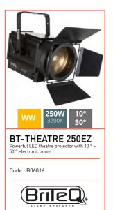
Optics: 1x250W 3200K COB LED Opening zoom angle: 10° to 50° Brightness of 1500 to 7735 Lux at 4m Direct access to the dimmer and zoom Integrated control unit with LCD display with drop-down menu DMX IN/OUT with 3/5-pin XLR plugs POWER IN/OUT with powerCON plugs POWER IN/OUT with powerCON plugs Power consumption: 275 W heat sink and silent fan. Finish: Black Delivered with barndoor, filter frame Dimensions: 458 x 336 x 399 mm Weight: 8.9 kg
