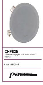
Power outputs : 35W RMS Impedance: 8 Ohms Components : 8" + 1 Sensitivity (1W/1m): 86 dB, +/-3dB Frequency response : 55-20 000 Hz Material : white plastic enclosure and magnetic grille Holding : 4 mouting clamp Dimensions : 260(diam) x 100 (H) mm Weight : 1,40 Kg
