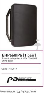
Power outputs : 7,5 / 15 / 30 / 60 W Voltage : 100 V 8 Ohms Components : 6,5" + 1" Sensitivity (1W/Iml: 90 dB, +/-3dB Frequency response : 70 - 20 000 Hz Material : Plastic enclosure and aluminium grille Holding : Wallmount bracket Connectors : Waterproof cable on gland IP55 Power rotary knob :  $60W 8\Omega // 7,5 / 15 / 30 / 60 W 100V$
