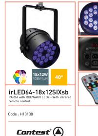
18x12W six-colour RGBWA + UV LEDs Beam opening: 40° Light intensity: 3350 Lux at 3 m Infrared remote control Digital display with drop-down menu Input and output on IEC plugs Modes of operation: 2-9 channel DMX, Fixed colours, Step or Fade programs, Auto mode with sound sensitivity, Slave Mode, Editing and playback of a 20-step program Power consumption: 240 W Power supply: AC 100/240V - 50/60Hz DMX input and output Black aluminium housing Dimensions: 340 x 270 x 220 mm Net weight: 5.4 kg
