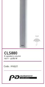
Power rating: 80 W RMS Available power: 80 W / 40 W at 100 V Speaker: 8 x 2.5 inches Frequency response: 250 Hz -15 KHz Sensitivity (1 W @ 1 m]: 97 dB Aluminium body and grill, Ingress protection: IP44 (weather-resistant) Dimensions: 104 x 73 x 690 mm Weight: 3.34 kg
