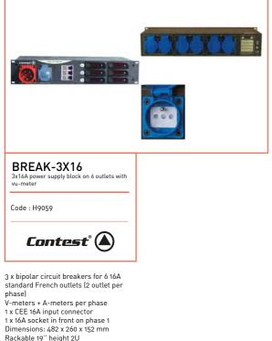
Rackable 19'' height 2U Power supply: 400V - 50 Hz (3P+N+E) Weight: 3.8 kg
