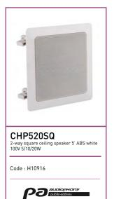
Power outputs: 5 / 10 / 20 WVoltage: 100 V / 8 ohmsComponents:  $4^{\circ} + 1/2^{\circ}$ Sensitivity (1W/1m): 89 dB, +/-3dBFrequency response: 90-18 000 HzMaterial: White plastic enclosure and metallic grille Holding: 4 mouting clamp Connectors: 4 contacts connector Drill hole dimensions:  $156 \times 156 mm$ Dimensions:  $190 \times 190 \times 80 (H) mm$ Weight: 1.3 Kg
