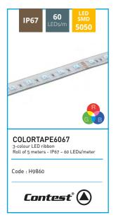
Trichromatic adhesive ribbon of 300 RGB LEDs for 5m Width: 12,5 mm Luminosity: 510 lumens/m Power required: 14.4W/m (72W for 5m) Voltage required: 24V (+ and -) Cuttable every 10 cm (6 LEDs) IP67: Full silicone sheath
