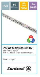
Ribbon of 300 4-colour RGBW LEDs for 5m Width: 12 mm Luminosity: 879 lumens/m Power required: 19.2W/m (96W for 5m) Voltage required: 24V (+ and -) Cuttable every 10 cm (6 LEDs) IP20: no protection no sealing
