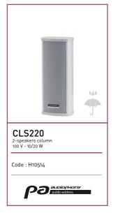
Power rating: 20 W RMS Available power: 20 W / 10 W at 100 V Speaker: 2 x 2.5 inches Frequency response: 250 Hz -15 KHz Sensitivity (1 W @ 1 m): 94 dB Aluminium body and grill, Ingress protection: IP44 (weather-resistant) Dimensions: 104 x 73 x 262 mm Weight: 1.4 kg
