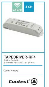
Mode of communication: 2.4GHz Power supply: 5 - 24V DC Intensity (max charge in amperes) : 5A x 4 (outputs) = 20A max Power rating: 100 W / 240 W / 480 W (5 V / 12 V / 24 V) Compatible remote control : REMOTERF-8RGBW Operating distance: 30m Dimensions: 175 x 44 x 30 mm Weight: 150 g
