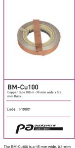
The BM-Cu100 is a-18 mm wide, 0.1-mm thick (1.8 mm<sup>2</sup> cross-section) copper tape insulated by a 0.05 mm Melinex band. Resistance +/- 10m $\Omega$ /m. Cables specially designed for induction loops where the loop must go under carpets or in places not suitable for conventional cables.
