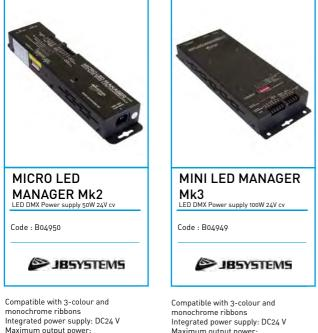
Maximum output power: - RGB : 16Wx3CH total 50W Integrated switch controller for: Master/Slave, 16 Colours, Musical, programs. 4-channel DMX operation Connection for wall controller LED WALL DIMMER and ON / OFF switch Power supply: AC230V - 50 Hz Dimensions: 332 x 70 x 40 mm Weight: 0.950 kg
