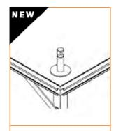
PLTEL-hc1 Attachment of guardrail to tray for PLTEL Code : H11109
