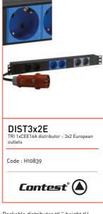
Rackable distributor 19 " height 1U Power input cable in 5G1.5mm<sup>2</sup> with a length of 2 m + Tetra CEE 16A plug 6 16A standard German sockets on the front (2 outlets per phase) Weight: 1.1 Kg
