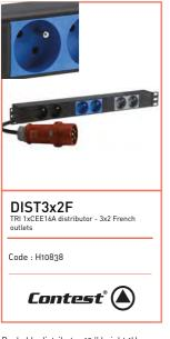
Rackable distributor 19 '' height 1U Power input cable in 5G1.5mm<sup>2</sup> with a length of 2 m + Tetra CEE 16A plug 6 16A standard French sockets on the front (2 outlets per phase) Weight: 1.1 Kg
