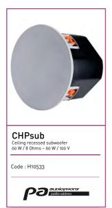
Power rating: 60 W RMS Available power: 60 W at 8 Ohms 60 W / 40 W / 20 W at 100 V Frequency response: 80 Hz -200 Hz Woofer: 8 inch Sensitivity (1 W @ 1 m): 95 dB Enclosed metal box Integrated passive filter External dimensions (diameter and depth): 295 x 215 mm Drilling diameter: 265 mm Net weight: 5 kg
