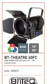
Optics: 1x 60W RGBW COB LED manual zoom: 10° to 50° 330 lux at 5m and 10°, 77 lux at 5m and 40° Integrated control unit with LCD display with drop-down menu DMX IN/OUT with 3-pin XLR plugs POWER IN with 1 m cord with plug Power supply: 100-240V/50-60Hz Power consumption: 62 W Dissipation fan Finish: black Delivered with barndoor filter frame Dimensions: 241 x 196 x 173 mm Weight: 3.6 kg
