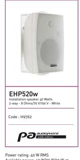
Available power: 40 W/20 W/10 W at 100 V – 20 W/10 W/5 W at 70 V 40 W at 8 Ohms Tweeter: 1" Woofer: 5" Frequency response: 80 Hz - 18 kHz Sensitivity (1 W @ 1 m): 89 dB Attachment: swivel bracket Dimensions: 270 x 187 x 165 mm Net weight: 3.4 kg Unit price – Sold by 2pcs
