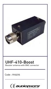
Gain from 9 dB +/-1dB Frequency range:  $500 \sim 950$  MHz Operating voltage: 8VImpedance  $50\Omega$
