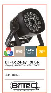
Optics: 8x18W RGBW LED Opening angle: 20° Integrated control unit with LCD display with drop-down menu DMX IN and OUT with 5-pin XLR plugs with waterproof plug POWER IN/OUT with original NEUTRIK Power Con® TRUE1 connectors Power supply: 100-240V/50-60Hz Power consumption: 129 W Waterproof fan Depressurisation valve with waterproof membrane Finish: cast aluminium painted black Dimensions : 305 x 273 x 192 mm Weightz : 5,28 kg
