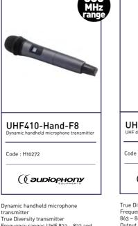
transmitter True Diversity transmitter Frequency ranges UHF 823 ~ 832 and 863 ~ 865 MHz Output power: 10mW (max.) 40 programmed frequencies with SYNC function LCD display: channel, battery level Power supply: 2 AA 1.5V batteries (not included) Average battery life: 10 hours Dimensions: 260 x 54mm diameter
