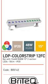
Optics: 12x4W RGBW 2-section LEDs Opening angle: 15° Integrated control unit with display with drop-down menu Power supply input/output on IEC plug DMX input/output on XLR 3-pin plug Power supply: 100-240V/50-60Hz Power consumption: 56 W Waterproofing level: IP20 Natural convection cooling Dimensions: 479 x 56 x 101/122 mm Weight: 2.2 kg
