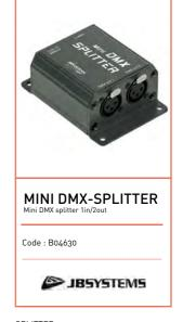
SPLITTER: 1 input and 2 DMX outputs BOOSTER: boost the signal Inputs: DMX XLR 3 Outputs: 2 DMX XLR3 Dimensions: 102 x 72 x 40 mm Weight: 0.24 kg
