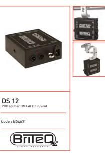
SPLITTER: 100% electrical insulation 1 input and 2 DMX outputs BOOSTER: boost the signal Bidirectional RDM compatible Inputs: DMX 3 and 5 XLR IEC 10A Outputs: 2 DMX XLR3 2 IEC 10A Dimensions: 130 x132 x 56 mm Weight: 0.95 kg
