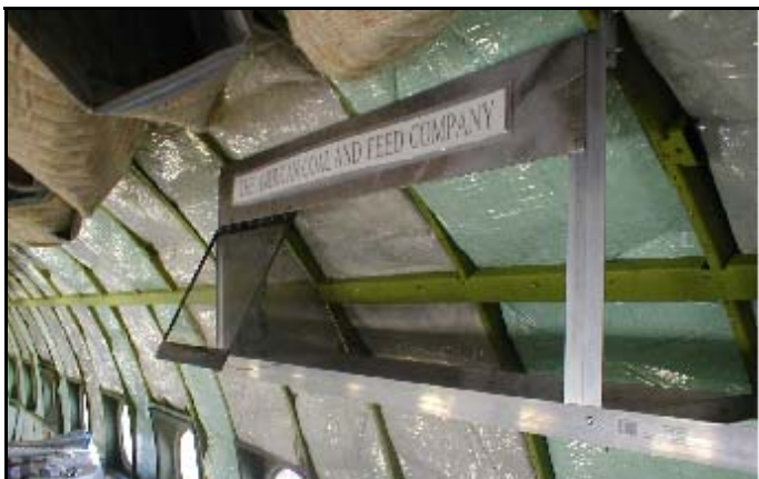
This photo taken on January 3rd, 2006. A prototype portion of the new display cases now being installed at Arcadia, Florida. This photo sent to us by Dexter Aviation, the contractor performing the work.
