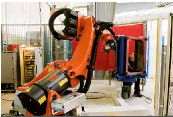
Robotic workstation for spot welding of wall-mounted cabinets
