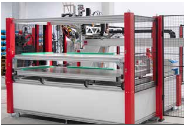
Center for glass gluing and cabinet door seal applications
