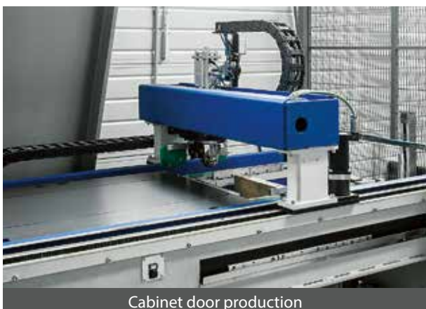
Combined machine - laser and punching
