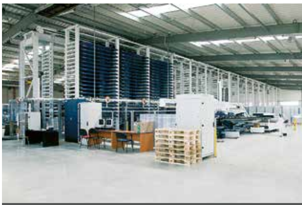
Automated warehouse for sheet steel and parts
