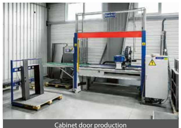
Deburring machine for cutout sections
