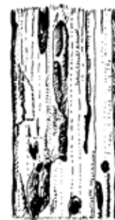
Carpenter ant damage to wood
