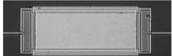
Figure 3. Mo/Cu bilayer with contact pads (on ends) and normal metal bars along the sides to suppress edge effects.
