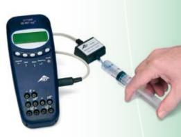
Measurement of absolute pressure as a function of volume
