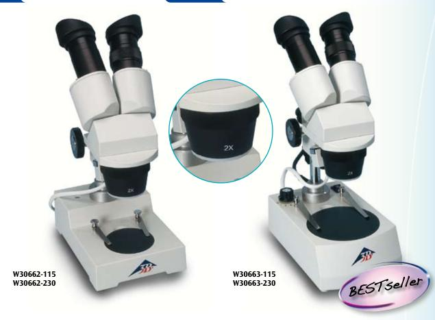
They can be used in numerous applications within the fields of biology and geology. Simply by rotating the objective from the 2x setting to 4x, the overall magnification can be set to 20x or 40x. With the aid of accessories, a magnification of up to 80x can be achieved. Model W30662 is lit from the top, while the W30663 can be illuminated by top light or by transmitted light, or by a combination of both. The large object stage of the W30663 also allows large objects to be observed.
