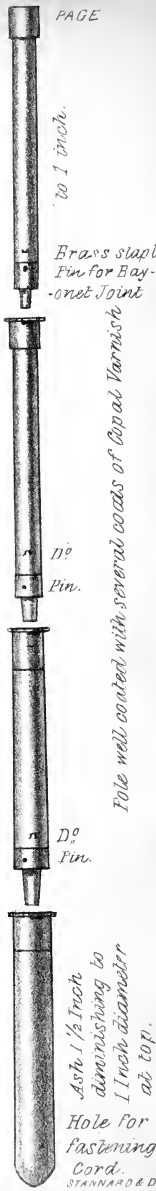
A. B. Either form for the Rake. All Iron Work coated with black varnish.
