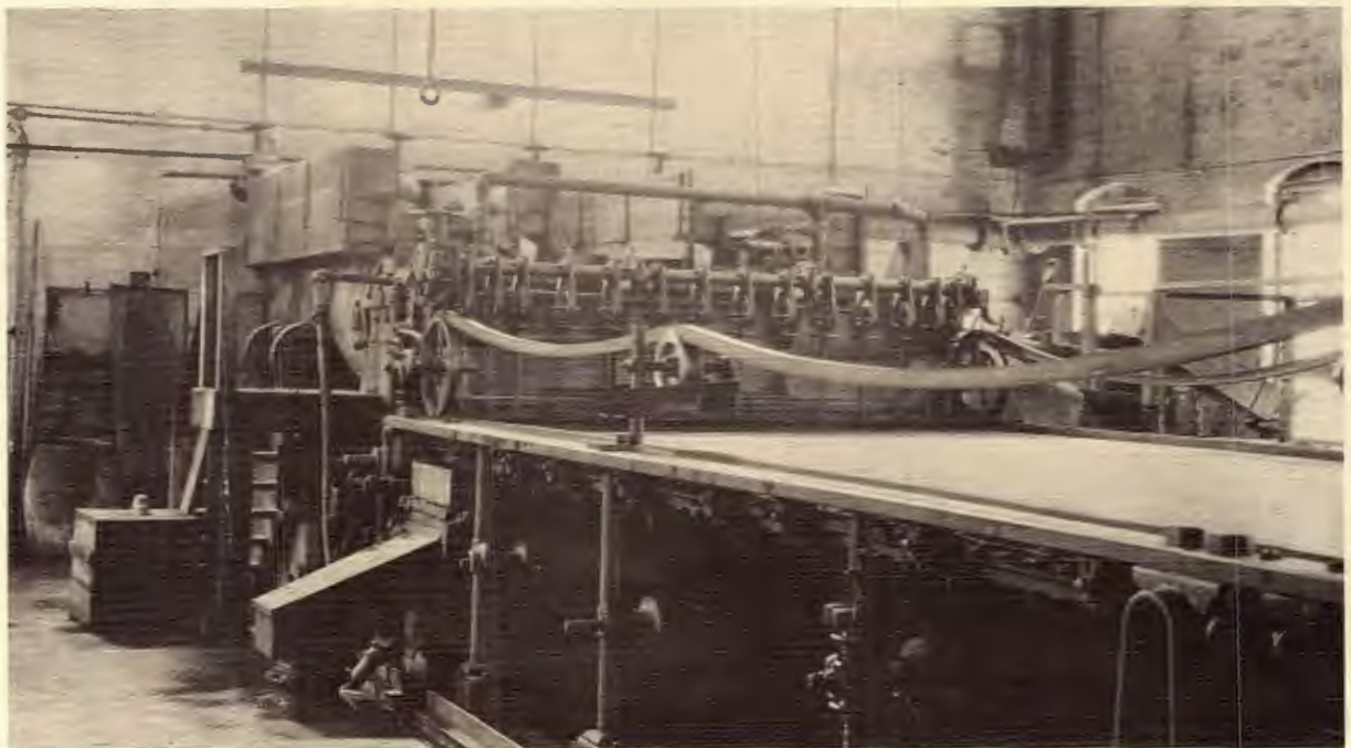
The wet end of Number 4 paper machine at Nekoosa illustrates the state of the art features of paper machines in 1915, i.e., deckle
