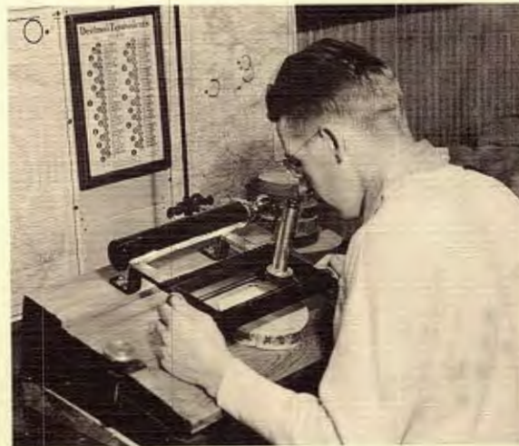
A quality paper requires quality raw materials. Here a wood technician evaluates the quality of the wood. A sample of a log is being microscopically examined.
