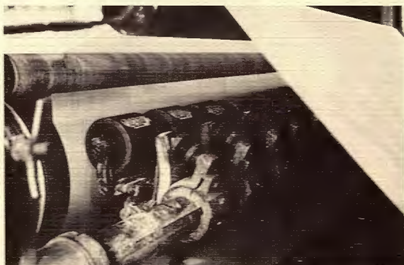
Watermarking rolls such as these, along with watermarking dandy rolls were used for putting the Nekoosa watermark into the paper. These are for Nekoosa Duplicator.
