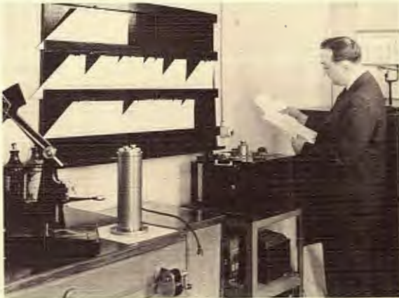
Testing apparatus for pre-testing Nekoosa papers is shown here. A brightness test is being made by the man in the photo.
