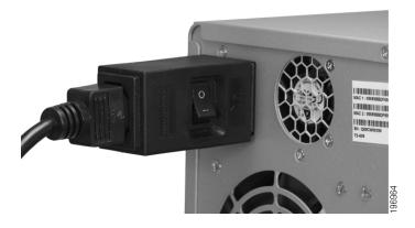
The following shows the DC inline switch module for the NSS 322.
