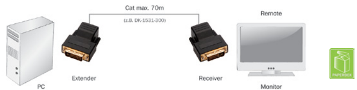
285694 / DS-54101 DVI-Extender via CAT5; single port
