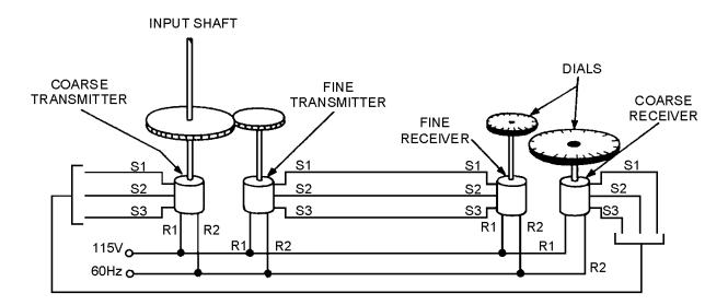
Figure 1-34.—Dual-speed synchro system.
