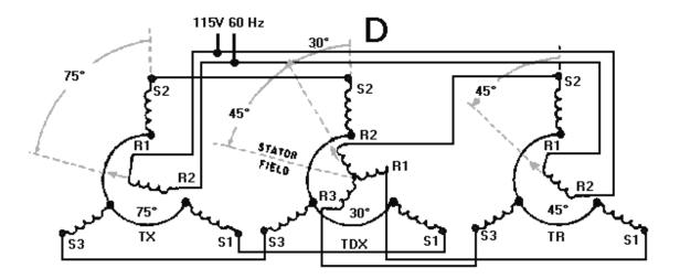
Figure 1-20D.—TX-TDX-TR system operation (subtraction).
