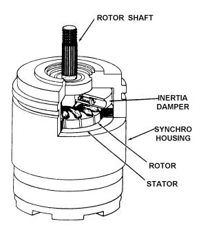
Figure 1-15.—Cutaway view of torque receiver with inertia damper.
