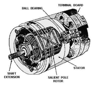
Figure 1-1.—Phantom view of a synchro.
