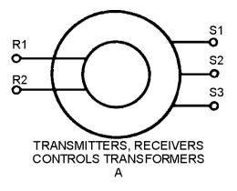
Figure 1-3A.—Schematic symbols for synchros.
