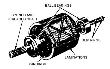
Figure 1-5.—Salient-pole rotor.
