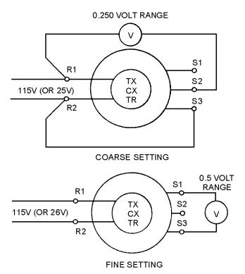
**ELECTRICAL-LOCK ZEROING METHOD** is perhaps the fastest. However, this method can be used only if the rotors of the synchros are free to turn and the leads are accessible. For this reason, this method is usually used on TRs.
