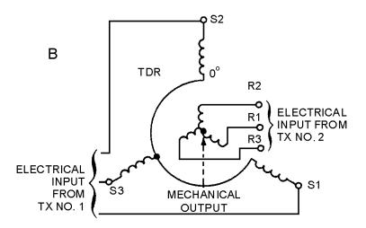
Figure 1-19B.—Torque differential receiver.
