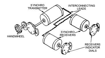
Figure 1-2.—Data transfer with synchros.
