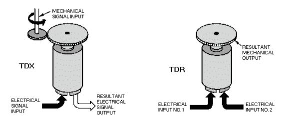
Figure 1-18.—Torque differentials.
