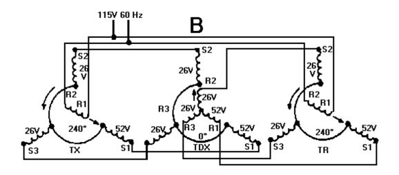
Figure 1-20B.—TX-TDX-TR system operation (subtraction).
