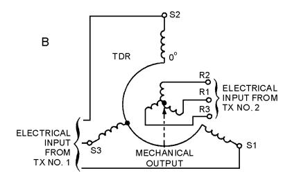
The **TX-TDX-TR SYSTEM** performs subtraction when the system contains standard synchro connections. Addition can also be performed with this system by reversing the S1 and S3 leads between the TX and the TDX, and the R1 and R3 leads between the TDX and the TR. Remember, this system works like a basic synchro system when the rotor of the TDX is on 0°; in this condition the TR rotor follows the TX rotor exactly.
