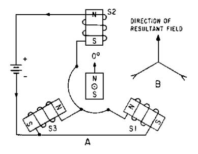
The **ZERO-DEGREE POSITION** of a synchro, transmitter is the position where the rotor and the S2 stator winding are parallel.
