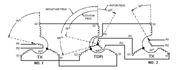
Figure 1-23.—TX-TDR-TX system operation (addition).
