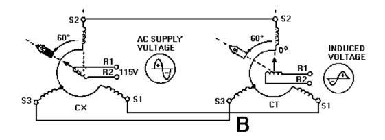
Figure 1-27B.—Control synchro system operation.
