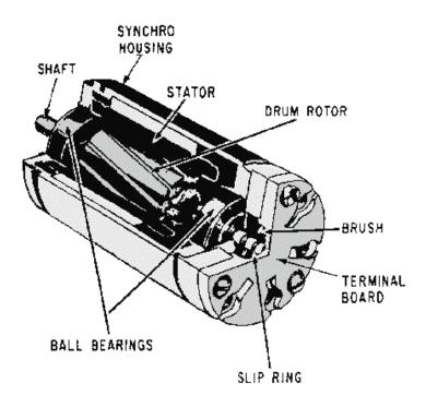
Figure 1-4.—Typical synchro assembly.
