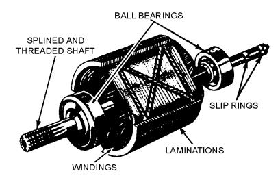
The **DRUM OR WOUND ROTOR** may be wound continuously with a single length of wire or may have a group of coils connected in series. This type of rotor is used in most synchro control
