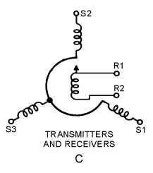
Figure 1-3C.—Schematic symbols for synchros.
