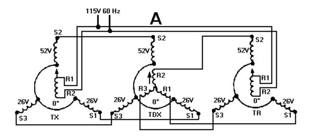
Figure 1-20A.—TX-TDX-TR system operation (subtraction).
