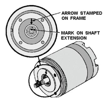
Figure 1-37.—Coarse electrical zero markings.
