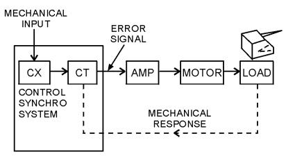
Figure 1-28.—A positioning servo system using a control synchro system.
