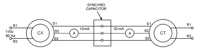
Figure 1-30.—The use of a synchro capacitor with a CT.
