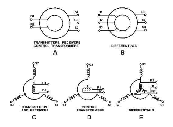
**SYNCHROS ARE CONSTRUCTED** like motors. Each contains a rotor, similar in appearance to the armature in a motor, and a stator which corresponds to the field in a motor.
