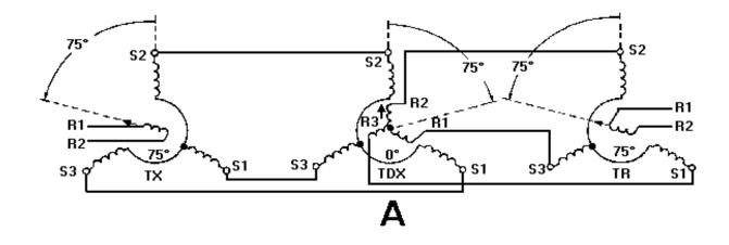
Figure 1-21A.—TX-TR system operation (addition).
