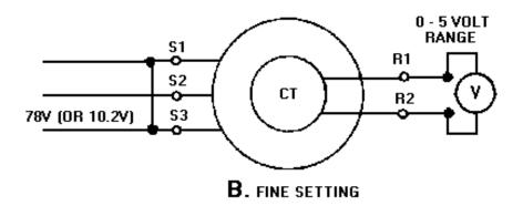
Figure 1-40B.—Zeroing a control transformer by the voltmeter method.
