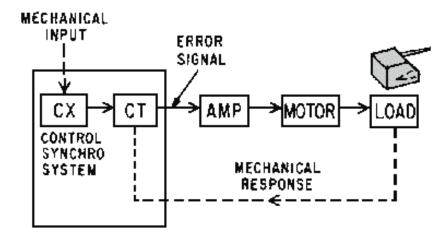
Figure 1-27A.—Control synchro system operation.
