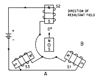
Figure 1-9.—Operation of three electromagnets spaced 120° apart.
