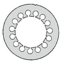
Figure 1-7B.—Stator lamination.
