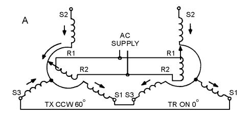
**REVERSED ROTOR CONNECTIONS** are common problems in new or modified synchro systems and should not be confused with the deliberate reversal of the stator connections. The reversal of the R1 and R2 connections on a synchro rotor causes a 180° error between the synchro transmitter and the synchro receiver, but the direction of rotor rotation still remains the same.
