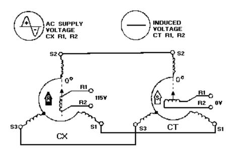
Figure 1-25.—CX-CT system operation with rotor in correspondence.
