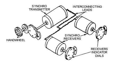
**TORQUE SYNCHRO SYSTEMS** are systems that use torque synchros to move light loads, such as dials and pointers.
