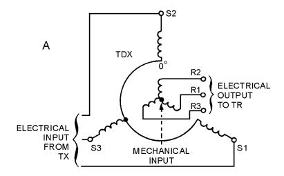
Figure 1-19A.—Torque differential transmitter.
