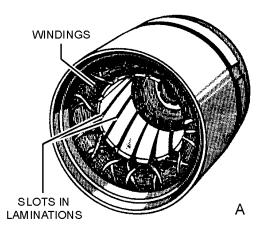
Figure 1-7A.—Typical stator.
