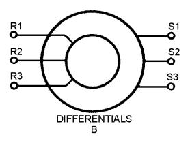
Figure 1-3B.—Schematic symbols for synchros.
