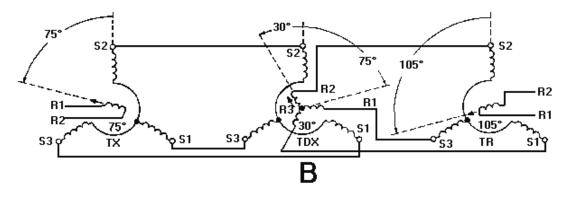
Figure 1-21B.—TX-TR system operation (addition).
