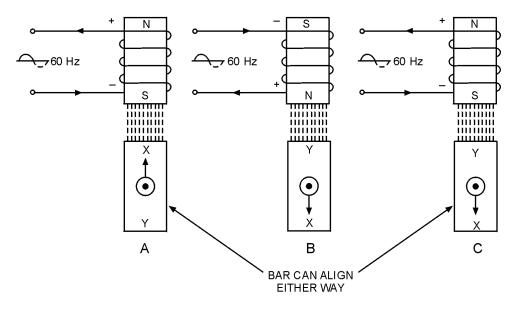
Figure 1-11.—Operation of an electromagnet with ac voltage.
