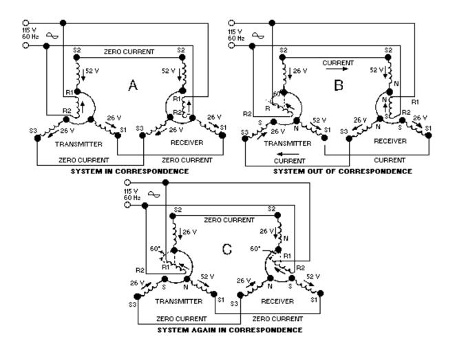
Figure 1-16.—A simple synchro transmission system.
