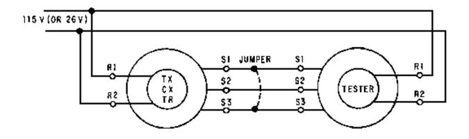
Figure 1-43.—Zeroing a synchro using a synchro tester.
