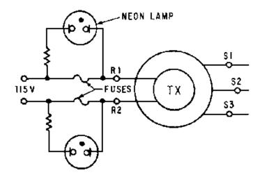
Figure 1-45.—Simple blown fuse indicator.
