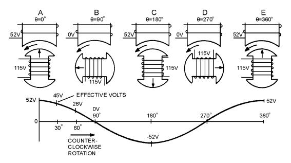
Figure 1-14.—Stator voltage vs rotor position.
