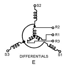
Figure 1-3E.—Schematic symbols for synchros.
