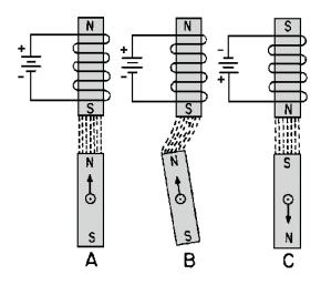
Figure 1-8.—Operation of an electromagnet with a bar-magnet rotor.
