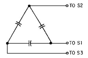
Figure 1-29.—The synchro capacitor.
