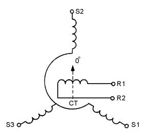
**ERROR SIGNAL** is the name given to the electrical output of a CT. The reason is that the electrical output voltage represents the amount and direction that the CX and CT rotors are out of correspondence. It is this error signal that eventually is used in moving the load in a typical servo system.
