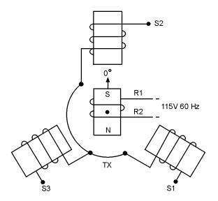
Figure 1-13.—Synchro transmitter.
