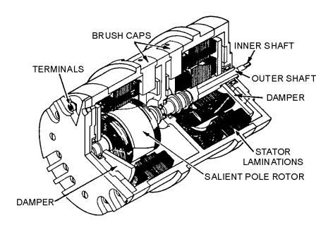
Figure 1-35.—Cutaway view of a double receiver.
