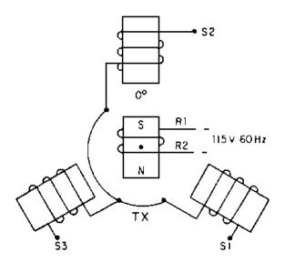
The **SYNCHRO TRANSMITTER (TX)** converts a mechanical input, which is the angular position of the rotor, into an electrical output signal. The output is taken from the stator windings and is used by a TDX, a TDR, or a TR to move light loads, such as dials and pointers.
