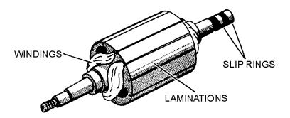
Figure 1-6.—Drum or wound rotor.
