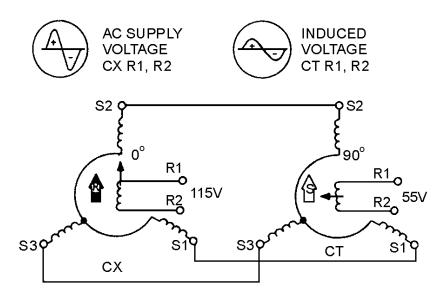
Figure 1-26.—CX-CT system operation with the CX rotor at 0° and the CT rotor at 90°.
