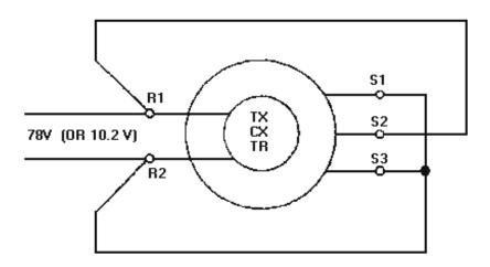
The **SYNCHRO-TESTER ZEROING METHOD** is potentially less accurate than the voltmeter or electric lock methods. This is because the dial on the tester is difficult to read and may slip from its locked position.
