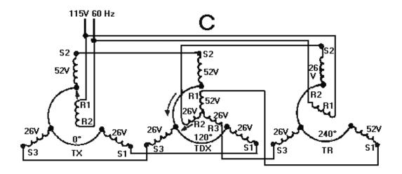
Figure 1-20C.—TX-TDX-TR system operation (subtraction).
