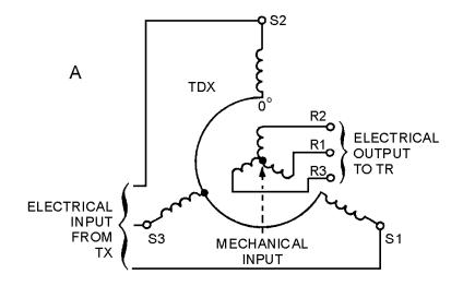
The **TORQUE DIFFERENTIAL RECEIVER (TDR)** is electrically identical to the TDX. The only difference in their construction is that the TDR has some form of damping. The real difference between the two differentials lies in their applications. The TDR has two electrical inputs, one to the rotor and the other to the stator. The output is the mechanical position of the rotor. As is the case with the TDX, the addition or subtraction function of the TDR depends upon how it is connected in the system.
