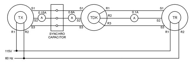
Figure 1-31.—The use of a synchro capacitor with a TDX.
