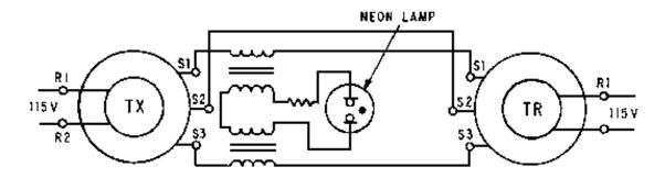
Figure 1-44.—Overload stator current indicator.
