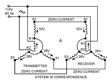
**SIGNAL** is defined as the angle through which a transmitter rotor is mechanically turned. This term has the same meaning as "transmitter's mechanical input."
