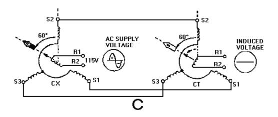
Figure 1-27C.—Control synchro system operation.
