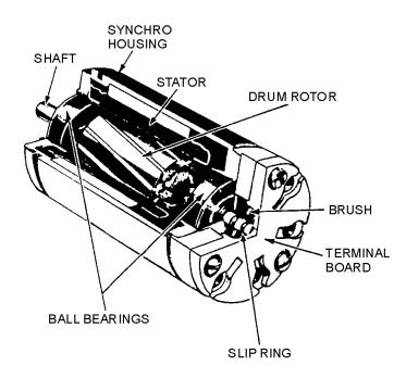
A **SYNCHRO ROTOR** is composed of either a single coil of wire wound on a laminated core or a group of coils wound in slots in a laminated core. The laminated core is rigidly mounted on a shaft that is free to turn inside the stator. Two slip rings are mounted on one end of the shaft to supply excitation voltage to the rotor. There are two common types of synchro rotors - the salient-pole rotor and the drum or wound rotor.
