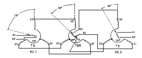
Figure 1-22.—TX-TDR-TX system operation (subtraction).
