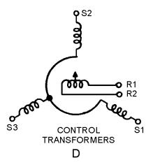
Figure 1-3D.—Schematic symbols for synchros.
