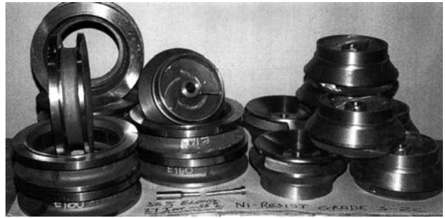
Pump impellers and vertical parts. Pumps made from these parts were for marine service but they could have been used in many different environments and industries. Ni-Resist D-2C. (The Taylor Group, Larbert, U.K.)
