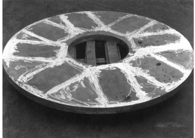
Unpolished lapping wheel. Weight 1070 kgs (2350 lbs). Ni-Resist D-2. (Macaulay Foundry, Berkeley, California, U.S.A.)
