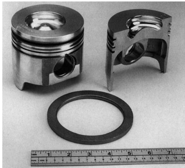
Aluminum alloy piston for a truck diesel engine with Ni-Resist 1 ring insert, cut-away view and Ni-Resist 1 ring prior to being cast in-place. (Zollner Pistons, Ft. Wayne, Indiana, U.S.A.)
